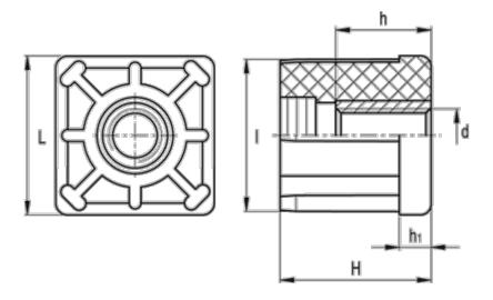
$\begin{array}{lll} d & = M20 \\ h & = 20 \\ H & = 45 \\ h1 & = 10 \\ Internal tube size = 47.0 \\ I & = 47.0 \\ L & = 50 \\ \end{array}$
